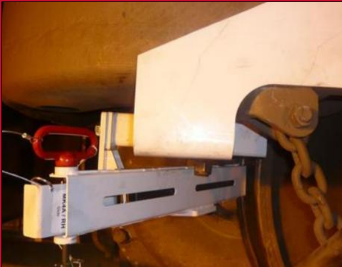
Locomotive Wheel Flange Solid Stick Lubrication
