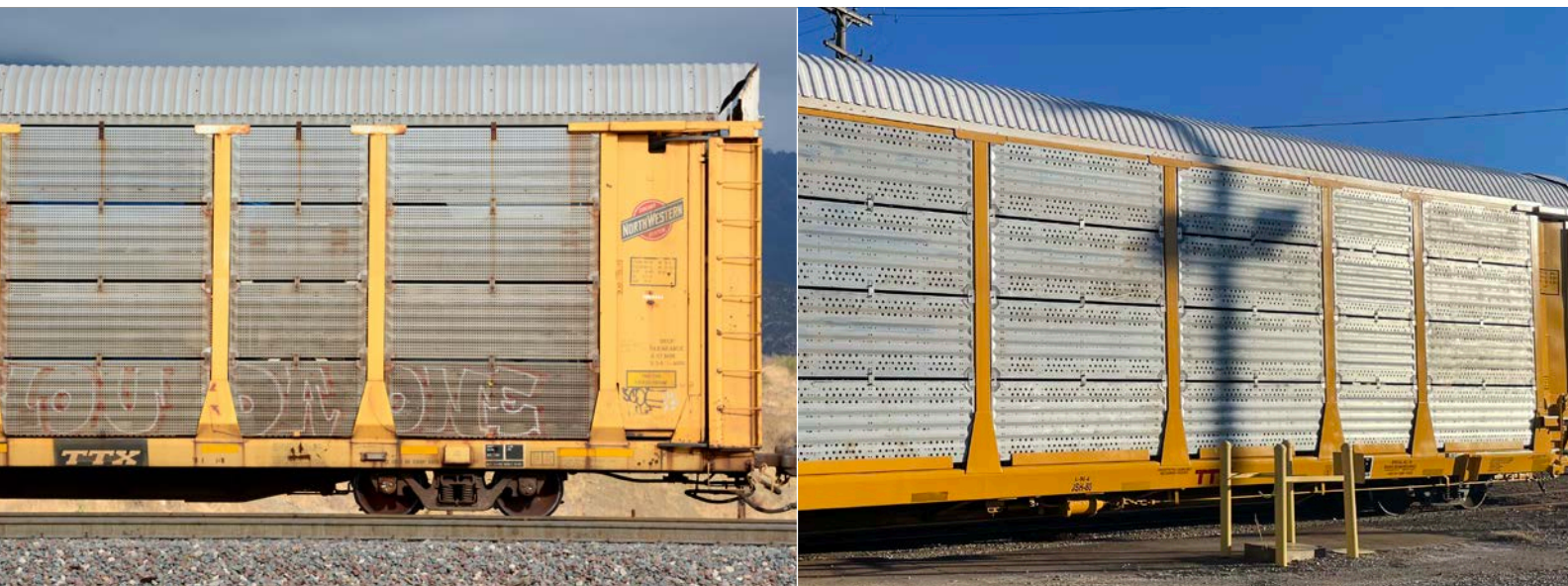
Older style side screens on auto racks, like the one at left, create aerodynamic drag. Newer versions, right, smooth airflow around the car. Chad Hewitt, left/Wayne Kennedy, right
