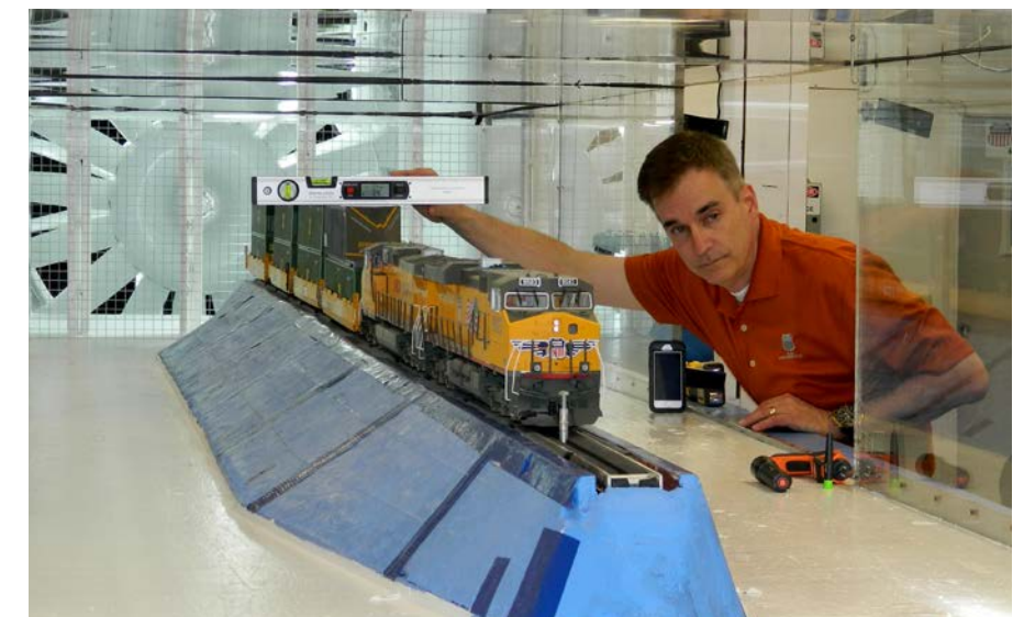
Brigham Young University designed this rail-centric wind tunnel that can test airflow on G-scale models. Here, Wayne Kennedy levels track sensors before a test. Wayne Kennedy
