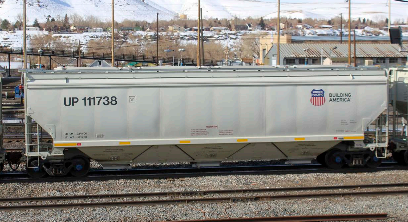
Union Pacific ordered 112 streamlined covered hoppers in 2018 after wind tunnel testing of G scale models proved the fuel saving potential of such aerodynamic design modifications, including enclosing the gaps between dump gates and new walkway supports that are one long continuous piece instead of individual brackets. Early testing of solid train sets of these covered hoppers, like this one at Green River, Wyo., showed that they reduced fuel usage by 4% to 6%. Andy Kirol
