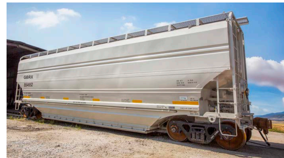
Greenbrier's Tsunami Gate covered hopper features aerodynamic refinements, most noticeable around the bottom gate, that reduce aerodynamic drag by 56%. Greenbrier
