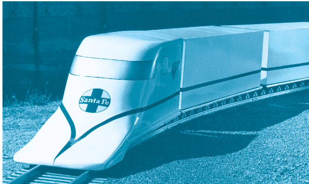
In 1969, Santa Fe developed a high-speed "coaxial train" concept. "It is a low-slung, low center of gravity train with a platypus-shaped lead unit to produce a desirable aerodynamic effect, and individually powered wheels spaced at four-foot intervals," the railway said. Santa Fe
