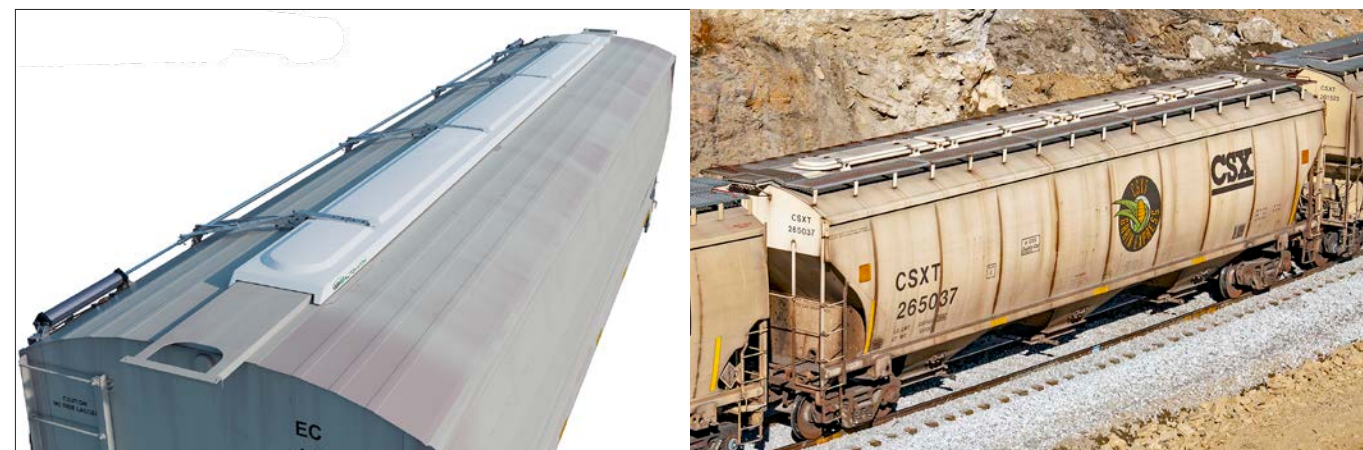
Car builder Trinity Rail has a prototype design, left, for an aerodynamic and automated covered hopper hatch called Ecofab. The hatch would eliminate the rooftop walkways that create aerodynamic drag on covered hoppers, like the CSX car at right. Trinity Rail, left; Robert J. Wise, right
